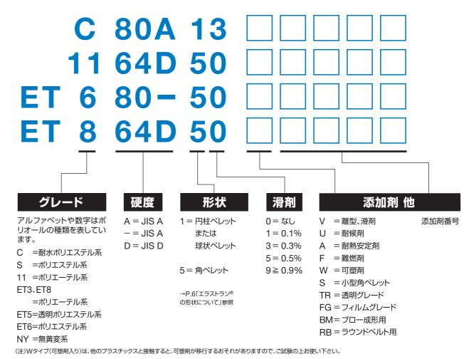
Hardness Pellet shape Lubi Grade 1 = Cylindrical or lentil-A = JIS A0 = nThe letter or number characterizes the base polyol - = JIS A shaped pellet 1 = 0.
